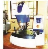
Polishing Machine for Polished Mount Preparation
